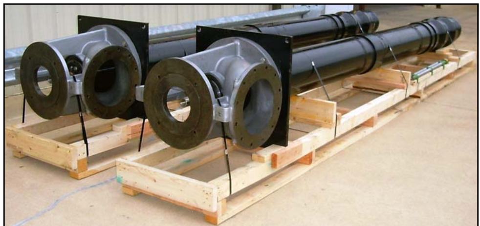
Hydroflo assembled short set pumps with 12" Discharge Heads.
